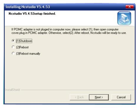
Press NEXT until finishing installation. Then turn off the computer and insert PCI control card into PCI slot of the computer. Start the computer again, the computer will automatically install driver program.
