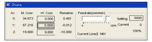
The system supplies the method for convenient setting and revising base point of work piece: Set current point as base point of work piece, that is to say, zero relative position of single axis. Move the cursor to coordinate display area of this axis and click left key of mouse, then coordinate of this axis can become 0. If needing set all current positions of three axes into 0, only need click in various coordinate areas.
