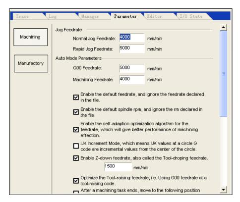
Manual speed: It includes manual high speed and manual low speed. These two values are used for movement speed under "jog" mode.
